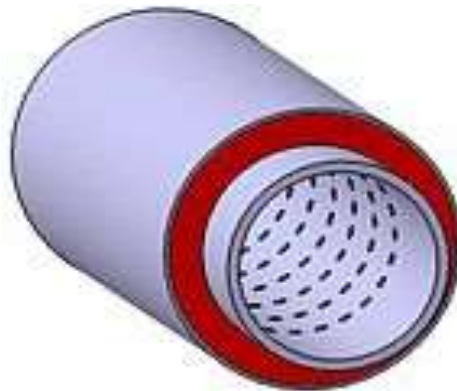
Figure 4.4 Absorber type muffler
